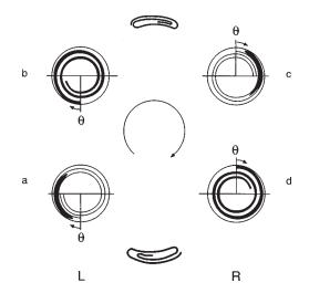
FIG. 78. Qualitative understanding of Duffing oscillator. (a) An elliptical open neighborhood in the left-hand well is (b) stretched out in the direction of motion during the first half period. When poured from the left-hand well to the right-hand well, it is squeezed into an elliptical neighborhood (c), which is a rotated image of (a). Stretching (d) and squeezing (a) continues.
