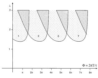
FIG. 84. Region in control-parameter space in which many bifurcations occur. The control parameters are the unstable Lyapunov exponent  $\lambda$  and the ratio of drive period to natural period. Each region can be identified by an odd integer, which is the local torsion of the node on which the bifurcation series is built.
