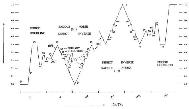
FIG. 83. Local torsion perestroika. Local torsion in a nonlinear oscillator changes in a systematic way as orbits are created on a direct horseshoe and annihilated from the reverse horseshoe.
