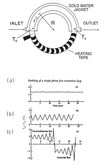
FIG. 77. Time series for temperature difference  $T_3 - T_9$  under three heat flow conditions. (a) Low heat flow: steady counterclockwise circulation. (b) Higher heat flow: oscillatory counterclockwise circulation. (c) Heating above instability threshold: chaotic behavior with unpredictable changes from counterclockwise to clockwise circulation. Top: experimental apparatus. Reprinted with permission from Creveling *et al.*, 1975. Copyright 1975 by American Institute of Physics.
