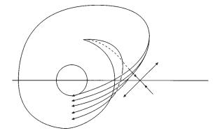
FIG. 67. Saddles and templates. A spiral saddle with one stable and two unstable directions organizes the rotational motion and is responsible for stretching. Its partner saddle with two stable and one unstable directions redirects the flow from its unstable direction to its stable directions, performing the squeezing (folding) that generates chaotic behavior.
