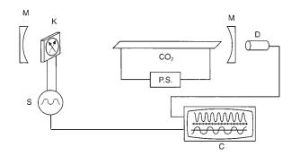
FIG. 1. Schematic representation of a laser with modulated losses.  $CO_2$ : laser tube containing  $CO_2$  with Brewster windows; M: mirrors forming cavity; P.S.: power source; K: Kerr cell; S: signal generator; D: detector; C: oscilloscope and recorder. A variable electric field across the Kerr cell varies its polarization direction and modulates the electric-field amplitude within the cavity.
