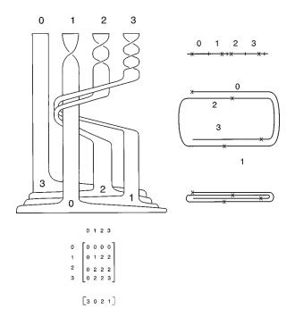
FIG. 80. Extended horseshoe. Template for a typical driven damped nonlinear oscillator is an extended horseshoe. The crosses show locations of period-one orbits.
