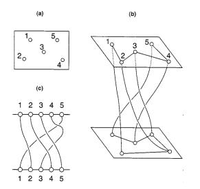
FIG. 65. (a) Five intersections of a period-5 orbit with a Poincaré section. (b) Flow lines from one section to itself. The flow deforms the phase space as indicated by the wrinkling of the segments connecting points in the Poincaré section. (c) Projection of the braid in (b) onto a plane  $R^2$ , keeping crossing information. The braid segments outline the template branches.
