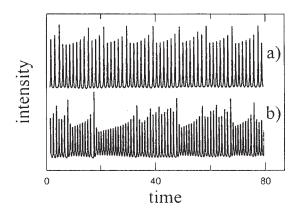
FIG. 73. Intensity output from an optically pumped molecular laser model under two operating conditions.
