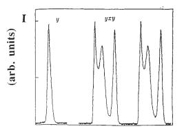
FIG. 64. Intensity trace for laser output, showing intervals of dead time between output spikes. These dead-time intervals make topological analyses difficult.
