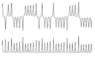
FIG. 75. Bottom: Segment of intensity data. Top: Conversion to amplitude data by implementing the algorithmic search for zero crossings.
